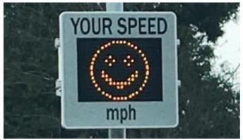
**Speed Indication Device (SID)** – The Parish Council has installed a SID on Ivetsey Road on the approach into Wheaton Aston. The device provides data on the speeds of vehicles entering the village.
